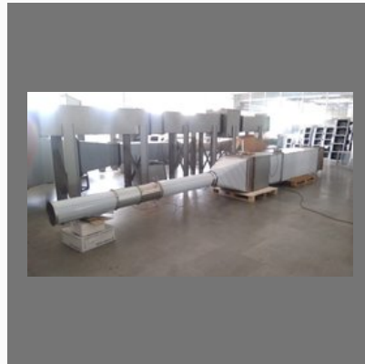
Air Filter Performance Test Rig
